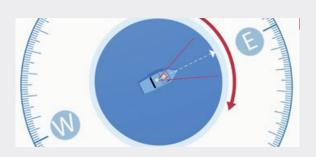
Dual antenna GNSS provides accurate heading with fast initialization time, even if the vessel is mooring.
