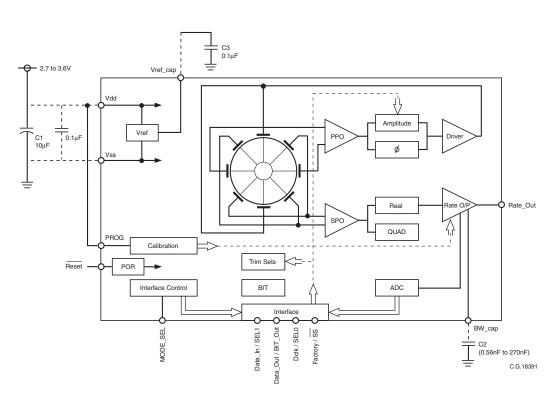
Figure 1.1 CRM100 Functional Block Diagram
