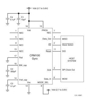
Figure 7.4 Peripheral Circuit - Digital Output (CRM100)
