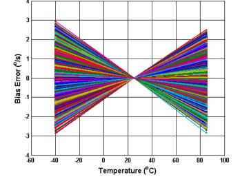
Figure 5.3 Analogue Normalised Bias Error (dps) vs Temperature
