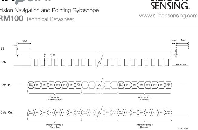
Figure 7.6 SPI® Timing
