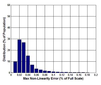
Figure 5.24 Analogue Maximum Linear Error (%) at 85°C
