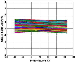
Figure 5.28 Digital Scale Factor Error (%) vs Temperature
